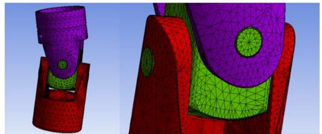
**Figure 7 Meshing in ANSYS WORKBENCH**
