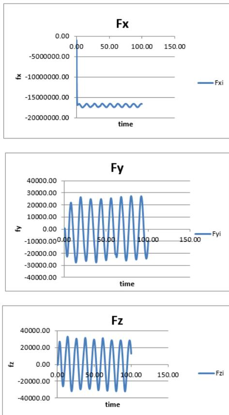
**Figure 6 Time varying forces on x, y & z coordinates on element 3**
