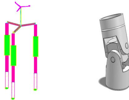
Figure 1 a)articulated tower b)universal joint
