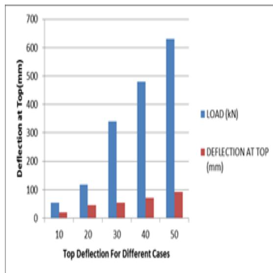
The graph of load Vs deflection for different number of stories considering p-delta effect under both Earthquake and wind loading is shown below :-
