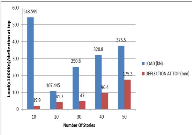
The graph of load Vs deflection for different number of stories considering without p-delta effect under both Earthquake and wind loading is shown below :-
