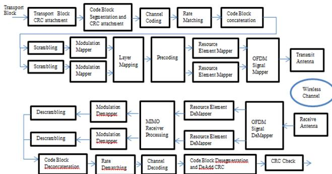
**Fig-2** PDSCH Transmitter and Receiver structure
