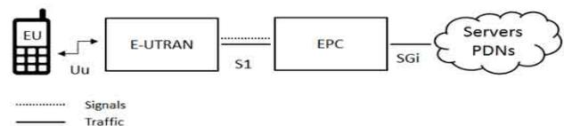
**Fig -1** LTE Network Structure
