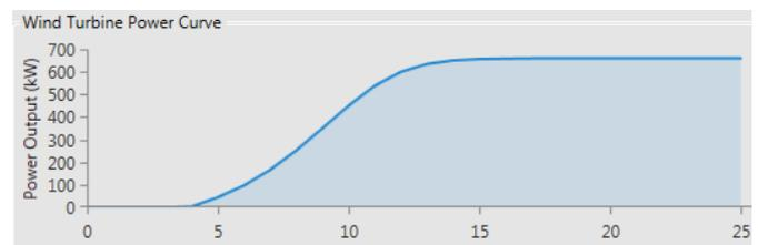
Fig -5: power curve of V-47 wind turbine
