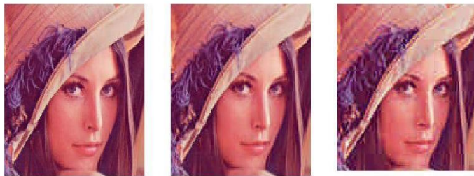
Figure.1 Illustration of compression using DCT: (a) Original Image compression ratio at (b) 88%, (c) 96%
