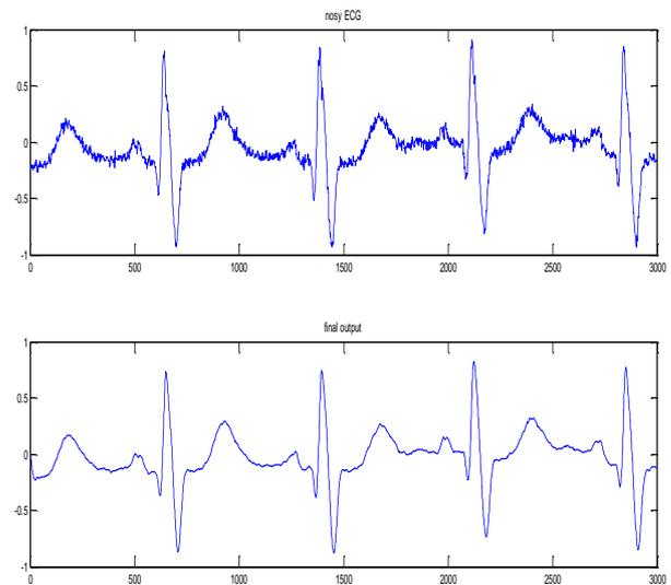
Fig- 8: results of LMS + low pass filter
