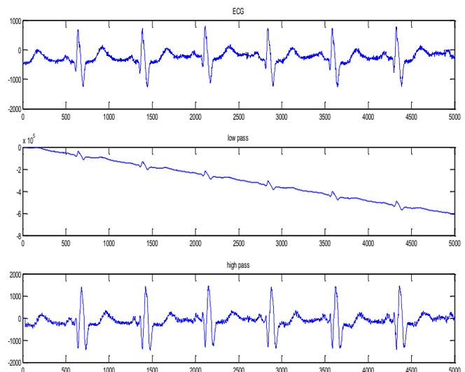
Fig -3: Results of Tompkins filter (a) noisy ECG (b) after Low pass filter (c) output of High pass filter
