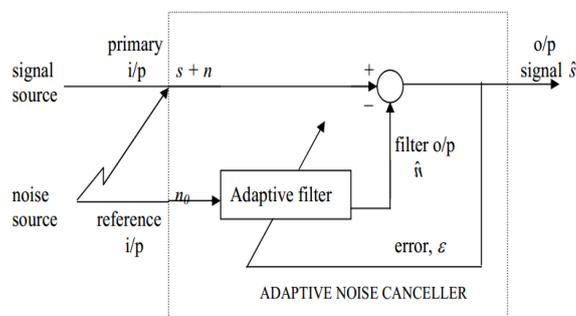
Fig- 5: Block diagram of Adaptive filter
