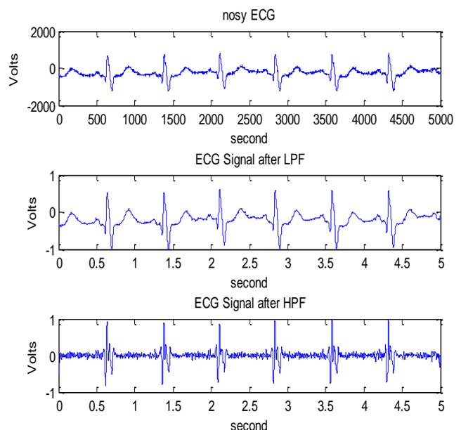
**Fig -2:** Output of Savitzky-Golay filter (a) noisy ECG signal (b) output of LPF (c) HPF
