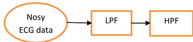
**Fig -1:** Savitzky – Golay filter (cascade connection of low pass and high pass filter)
