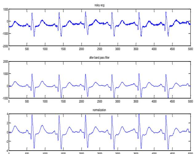
Fig -4: Results of Butterworth filter (a) noisy ECG signal (b) Output of Butterworth (c) Normalization
