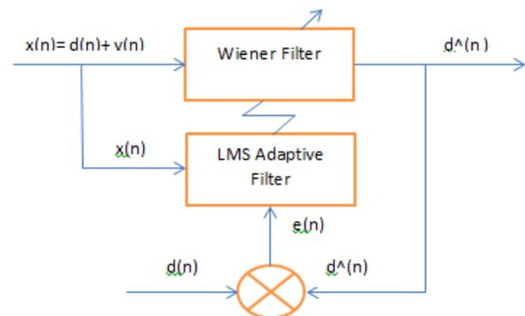
Fig- 6: Adaptive LMS filter block diagram
