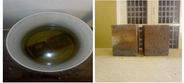
Fig-3 Acid attack
