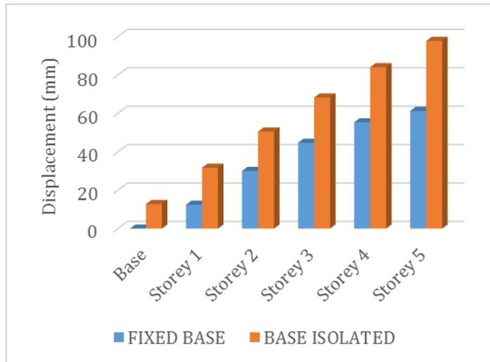
Fig-9: Storey displacement for fixed base and Base isolated building
