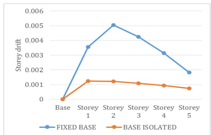
Fig-12 Storey drift for fixed base and Base isolated building
