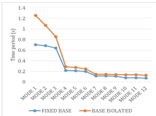
Fig-10 Time period for fixed base and Base isolated building
