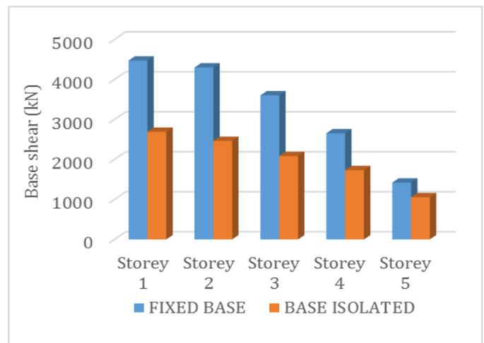
Fig-11 Base shear for fixed base and Base isolated building
