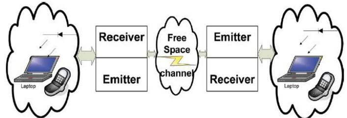
Figure 3: Overall Block Diagram of VLC
