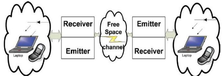
Figure 3: Overall Block Diagram of VLC
