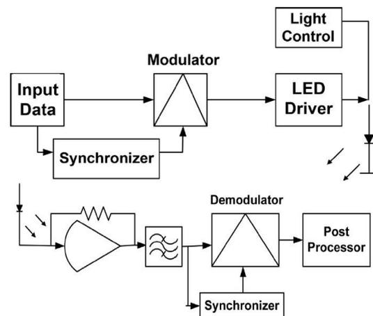
Figure 4: Transmitter & Receiver Blocks
