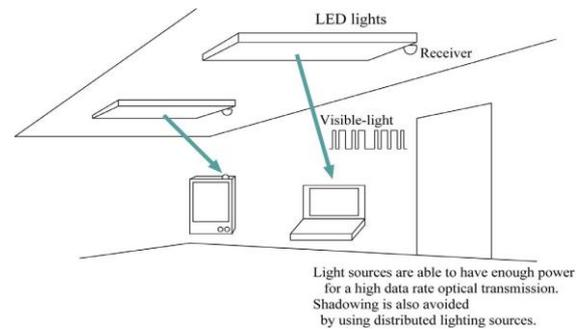
**Fig.5 Visible-light communication system utilizing white LED lights**
