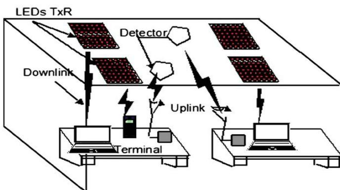
Figure 2: VLC system for indoor application
