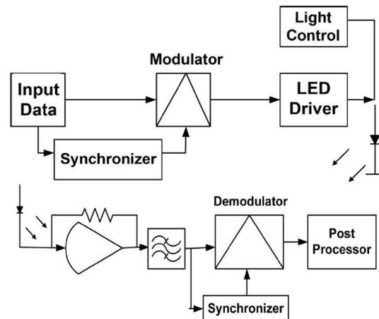
Figure 4: Transmitter & Receiver Blocks
