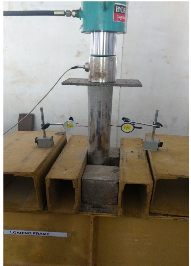
Fig-10. Test setup for Lateral deformation
