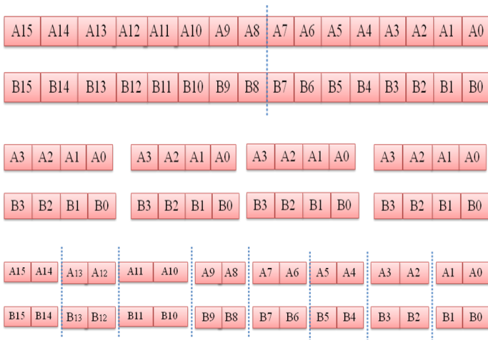
Fig - 9: Modified Vedic multiplication of two 16-bit numbers.
