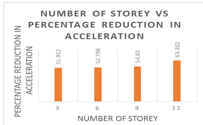
**Fig. - 4:** Graph showing number of storey Vs percentage reduction in acceleration
