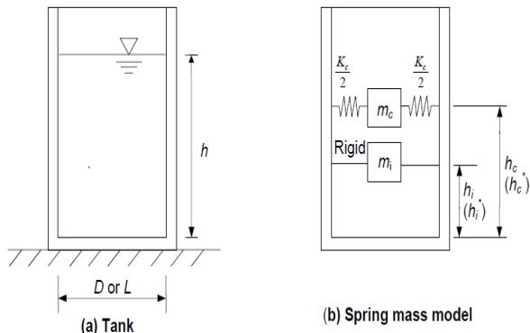
**Fig-1:** Spring mass model for rectangular tank
