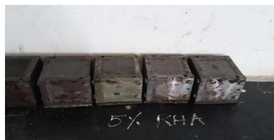
Fig.2 Moulds filled with cement mortar
