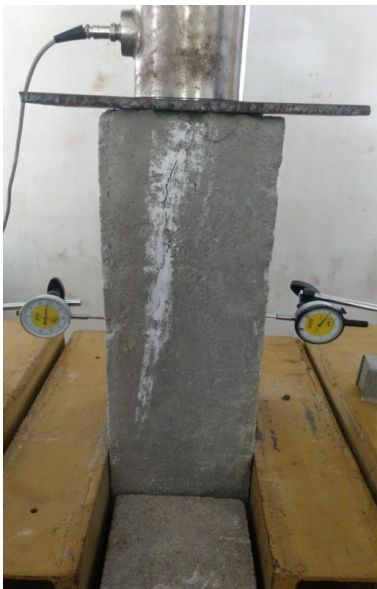
Fig 14 Mode of Failure
