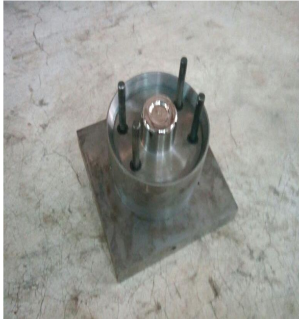
Figure 6.2.3 (a) Punch of the mould
