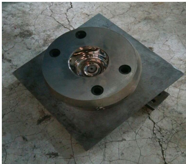
Figure 6.2.4 (b) Cavity half of the mould
