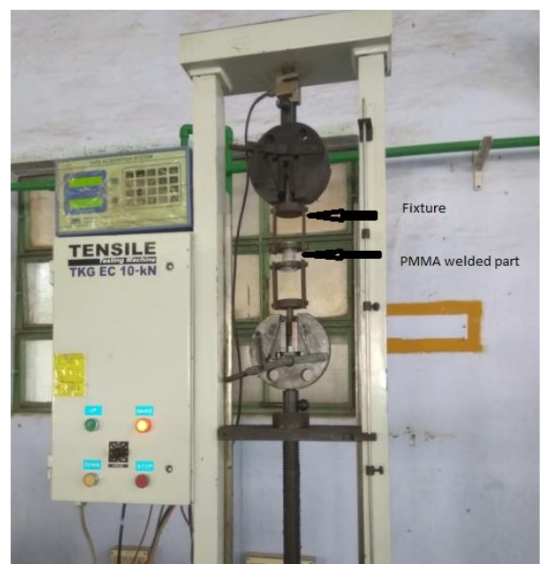
Figure 4 Tensile testing of PMMA welded specimen
