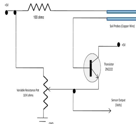
**FIGURE NO.3 Sensor design Equivalent diagram of soil moisture sensor**
