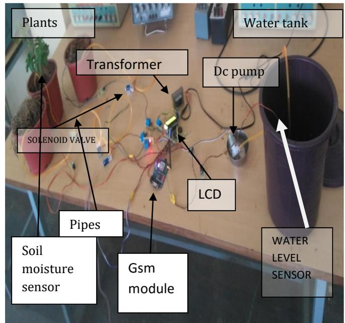
**Fig-4 ACTUAL EXPERIMENTAL SETUP**
