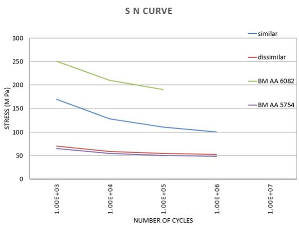
**Chart-3** S–N curves at R = 0.1 for butt joints tested along with base materials AA6082, A5754.
