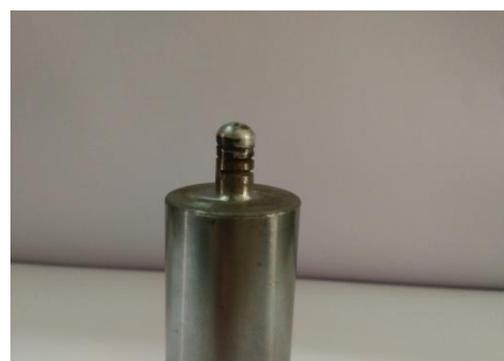
**Fig.1** FSW Tool Used
