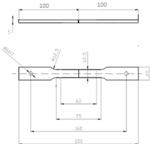
**Fig.2** Specimen geometry
