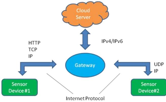
**Figure 3. Device-to-gateway communication model diagram.**
