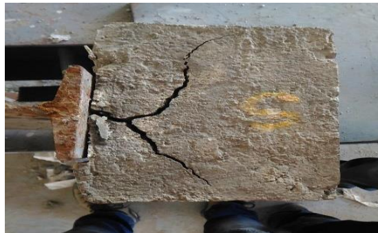
Fig.10 - Failure mode of channel shaped shear connector
