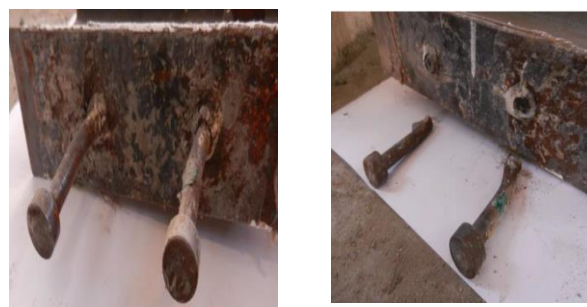
Fig.8 - Failure mode of stud shaped shear connector
