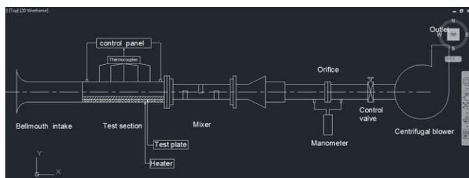
**Fig 7: Standard Experimental Setup**
