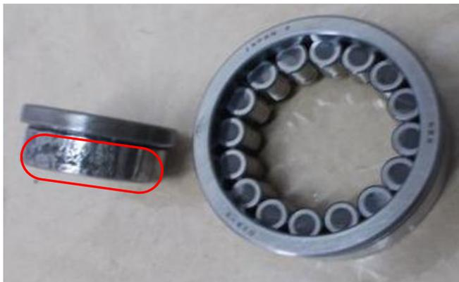
**Figure -1:** Damaged of the Inner race of the counter shaft bearing
