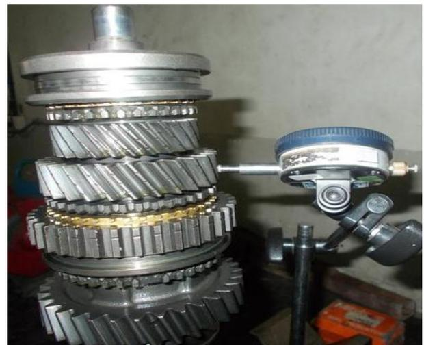
**Figure -2:** Gears clearances and the foreign particles accumulated on the magnetic brush
