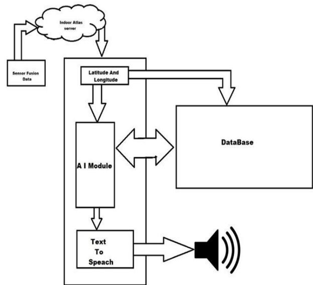
Figure 2.1: Block diagram of navigation assistant
