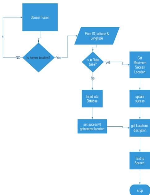
Figure 2.2: Flow chart of AI module
