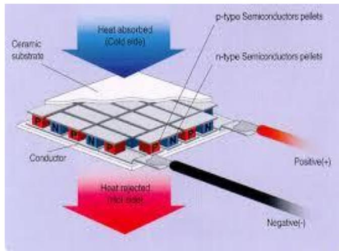
Fig -1: Thermoelectric Module
