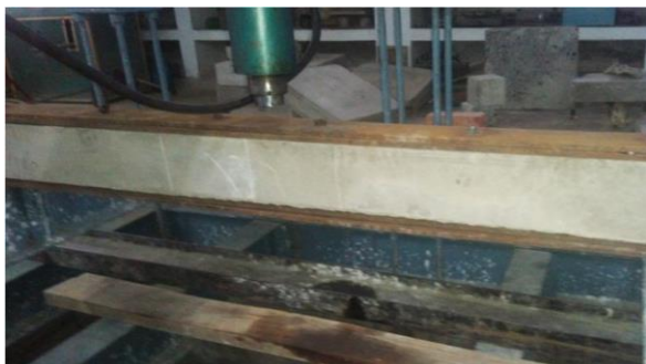
Fig.5: Beam two is retrofitted with double plates top and double plate base of the beam
