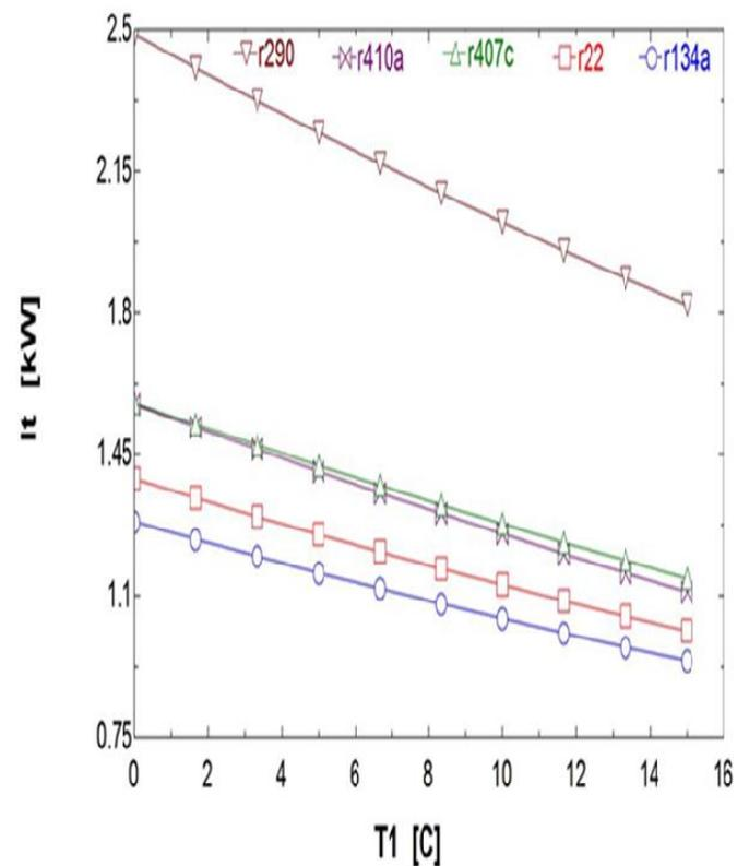
Fig 6 Evaporator temperature and Total irreversibility
