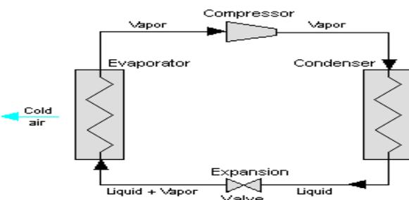
Fig 2 Component of vapour compression refrigeration system
