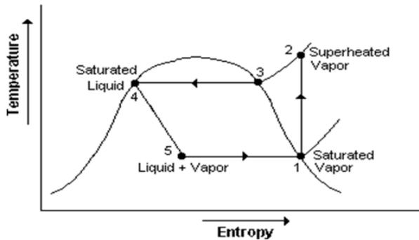
Fig 1 T-S Plot of Vapour compression cycle
