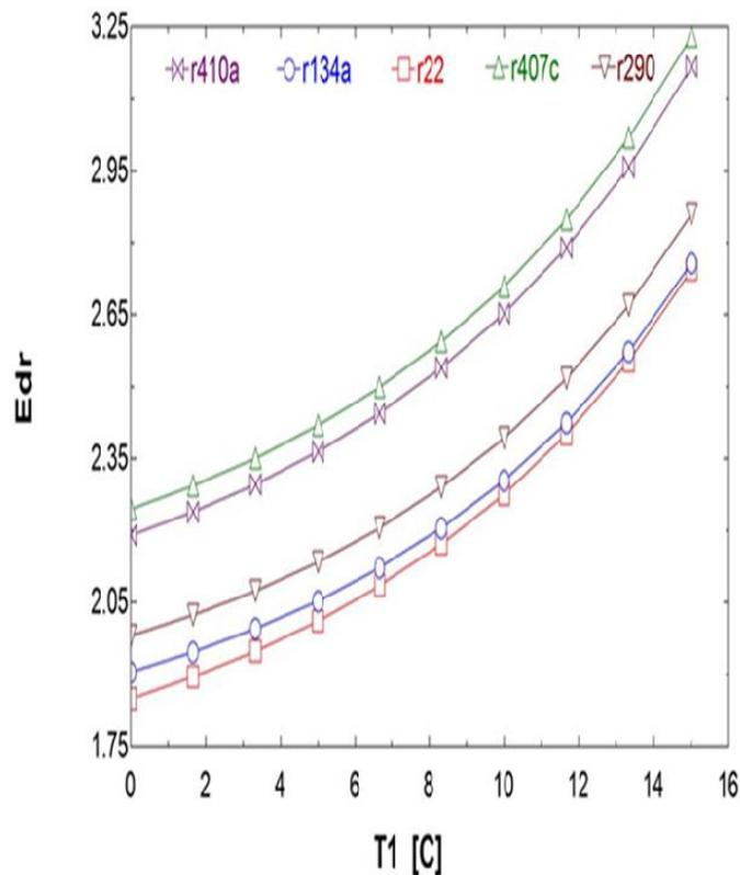
Fig 4 Evaporator temperature and Exergy destruction ratio
