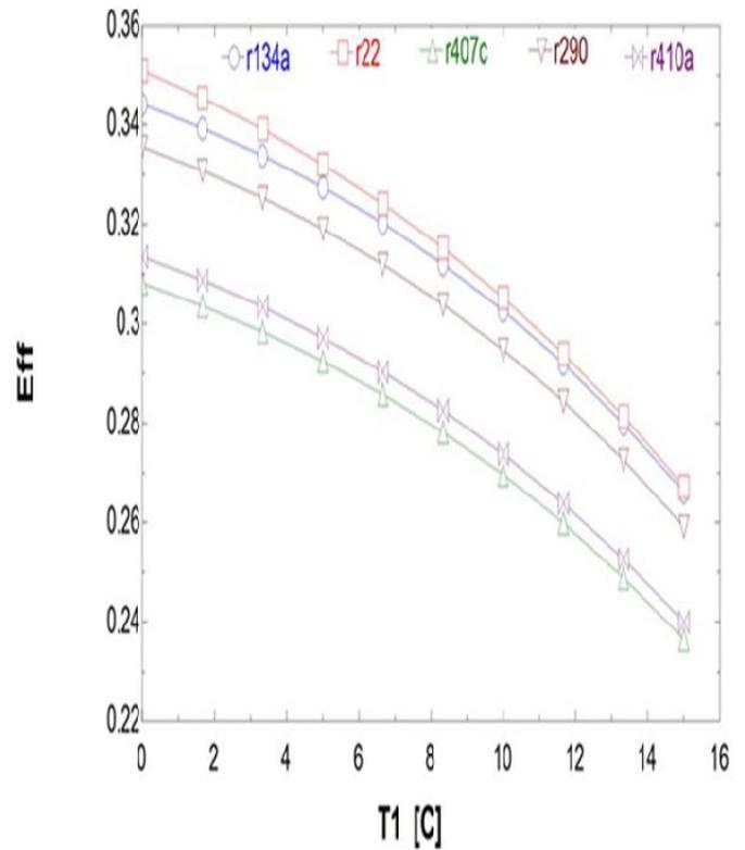
Fig 5 Evaporator temperature and Exergy efficiency
