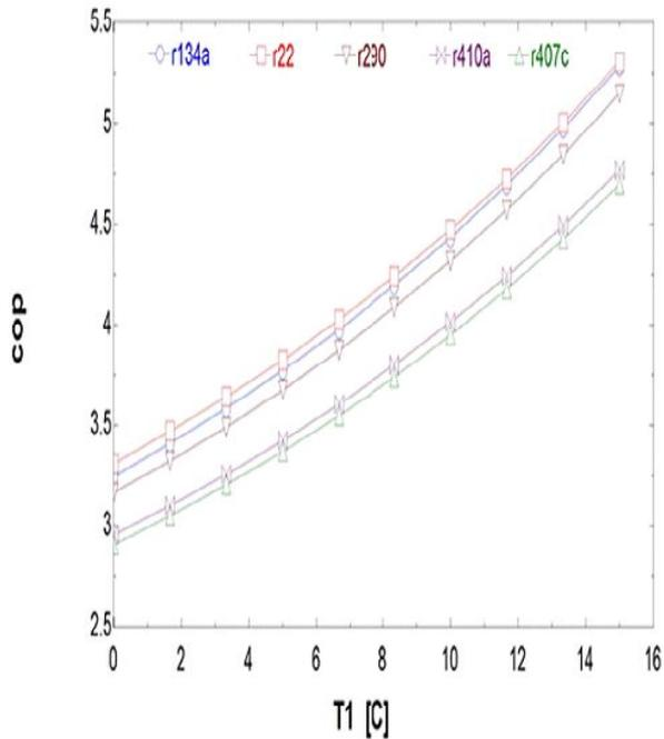
Fig 3 Evaporator temperature and coefficient of performance
