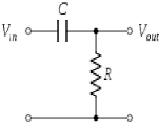
Figure 6. High Pass filter
