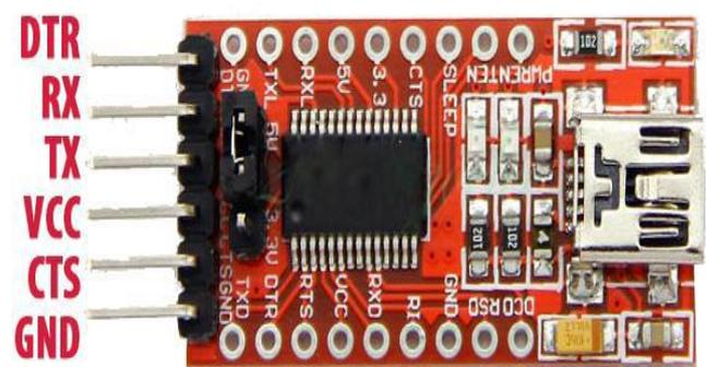
Figure1. FT232 pin diagram
