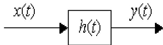
Figure 5. Block representation of transfer function
