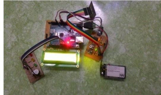
Fig-3: Image of Direct Photometry Non Invasive Bilirubin Device
