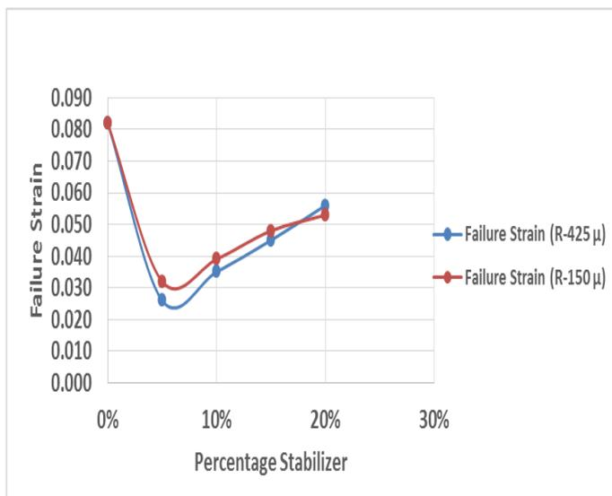
**Chart-4:** Comparison of failure strain of clay stabilized with various Percentages of tire scrap
