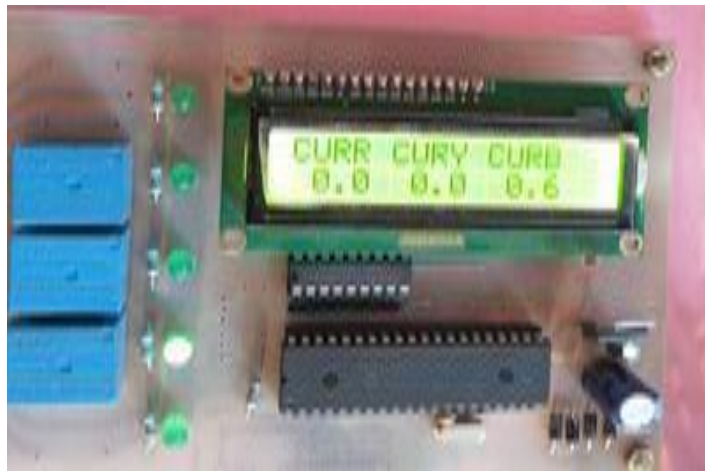
Fig -4: Three phase current indication.
