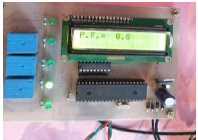
Fig -6: Less power factor indication
