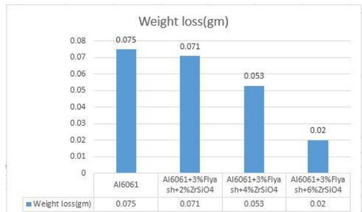
Fig 4.5 Weight Loss at 3Kg load
