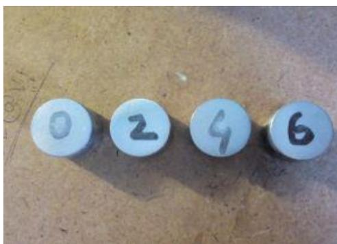
**Fig 3.2 Hardness test Specimens**
