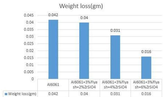
Fig 4.4 Weight Loss at 2Kg load
