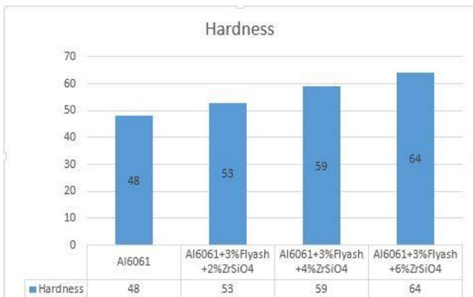
Fig 4.2 Hardness Vs Reinforcement
