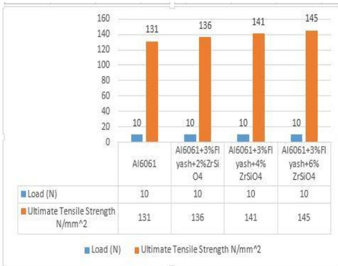
Fig 4.1 Load Vs Ultimate Tensile Strength
