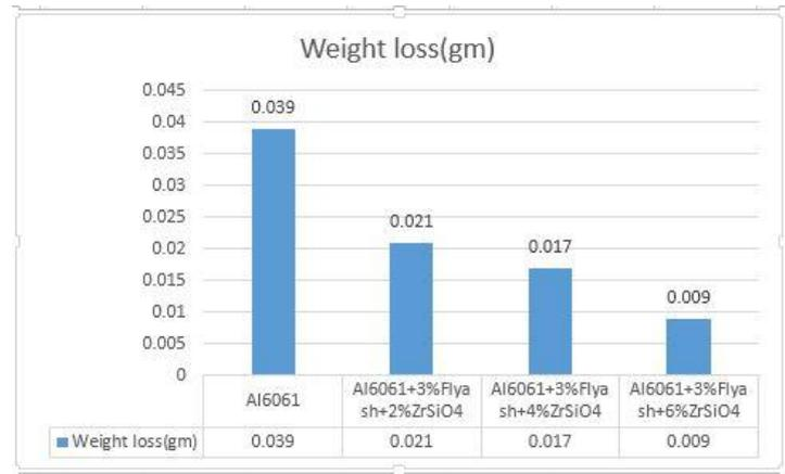
Fig 4.3 Weight Loss at 1Kg load
