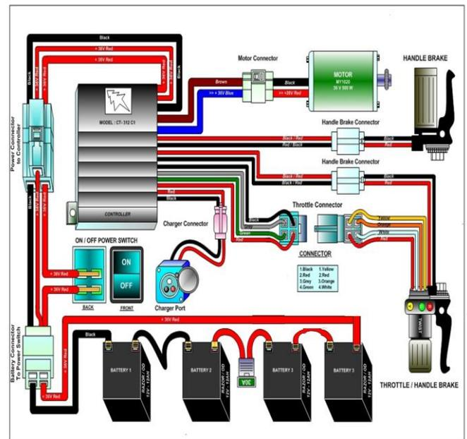
Fig -1: BLOCK DIAGRAM OF BIKE
