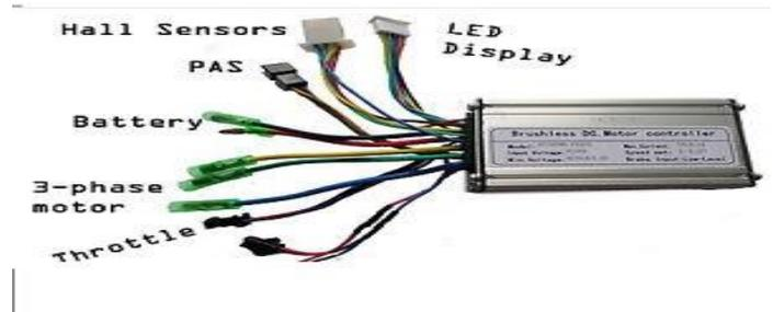
Fig -3: CONTROLLER CONNECTIONS
