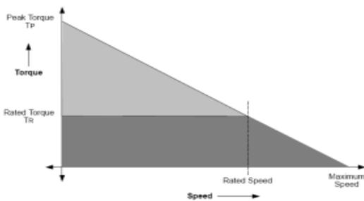
Fig -3: Speed torque characteristic
