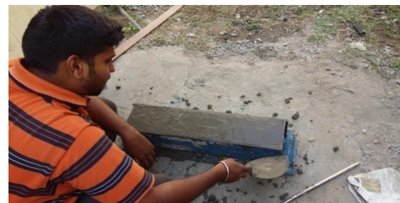
Figure 2: Casting of the specimen
