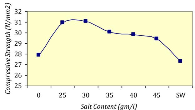
**Fig - 2:** Showing Average Compressive Strength of cubes at 7 Days Curing.
