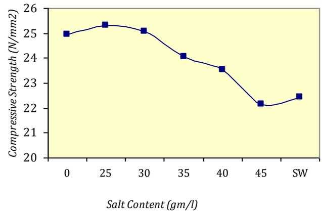
**Fig - 1:** Showing Average Compressive Strength of cubes at 3 Days Curing.
