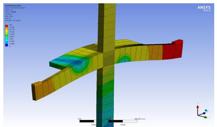
Fig -7: Cooling deformation of SRC Beam-Column joint (ISMB 175)
