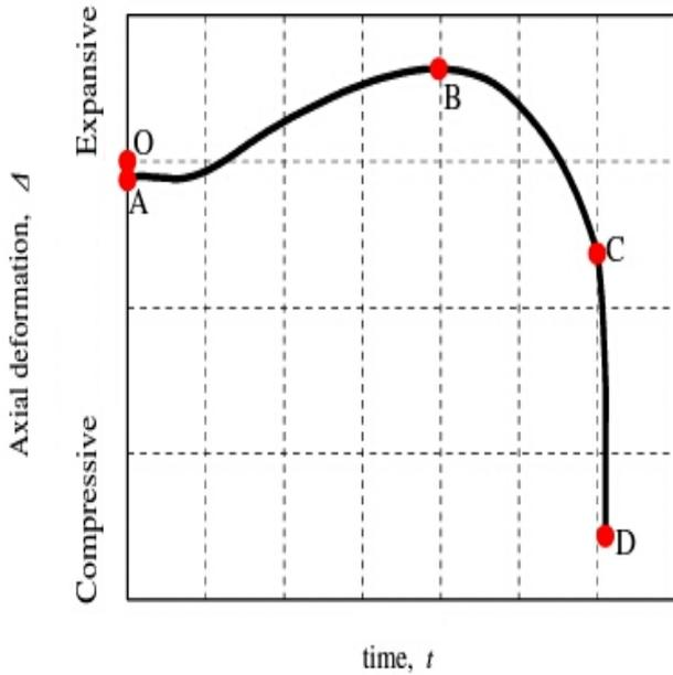
Fig -2: Typical SRC Column Axial Deformation versus Time Curve
