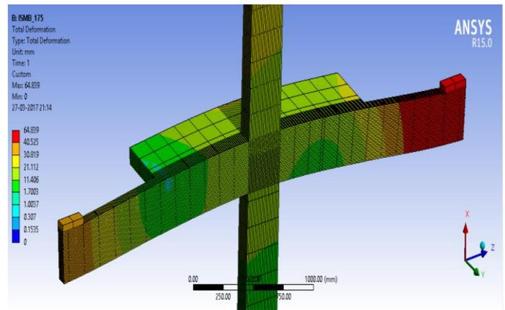
Fig -6: Heating deformation of SRC Beam-Column joint (ISMB 175)
