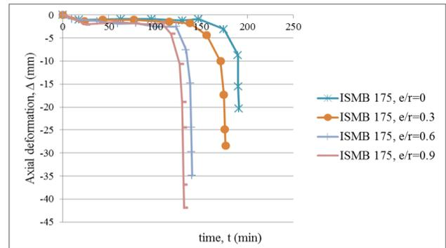
Fig -3: SRC Column (ISMB 175) Axial Deformation versus Time Curve
