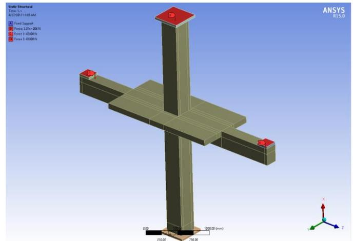
**Fig -4:** Modeling of SRC beam-to-column joint
