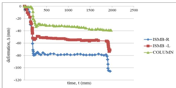
Fig -5: SRC Column (ISMB 175) Axial Deformation versus Time Curve
