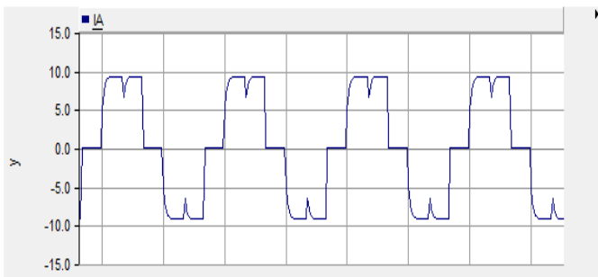
Fig-11 Output phase to ground voltage V_{AN} (120° mode)
