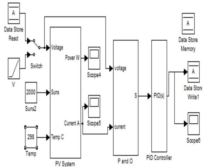
Figure.7. The proposed PID controller for PV module
