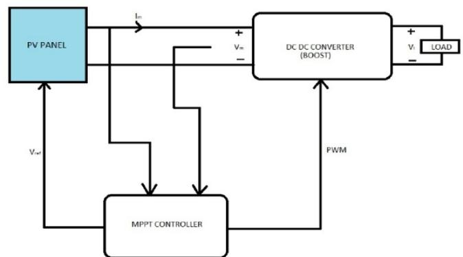
Figure.1. Block Diagram of PV Model
