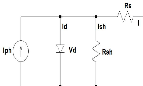
Figure.2. Solar cell equivalent circuit
