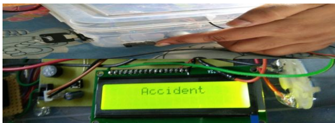
Fig-14: An image when limit switch is pressed,that is attached on the front side of the vehicle.It is used to detect accident when any of the object hits on the front side of the car.The message will be sent to pre-recorded number on the accident detection using GPS and GSM along with the location of vehicle.
