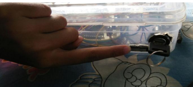
Fig-5: An image showing the working of seatbelt. Limit switch is used to represent seatbelt. Unless and until you connect seatbelt (press limit switch) the car engine will not start and car won't go ahead.
