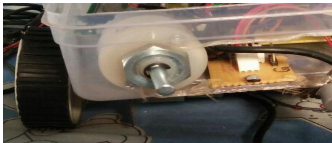
Fig-12: An image of motor (wiper) which will start automatically without need of manual intervention as soon as rain is detected.
