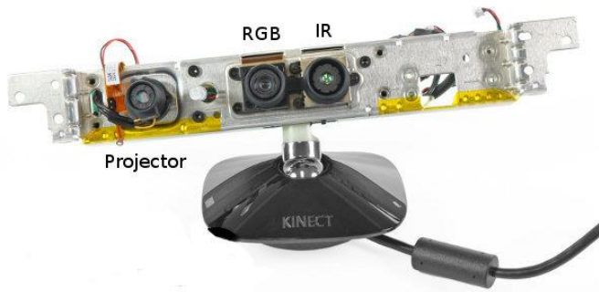
Figure 5: Kinect consists of Infra-red (IR) projector, IR camera and RGB camera
