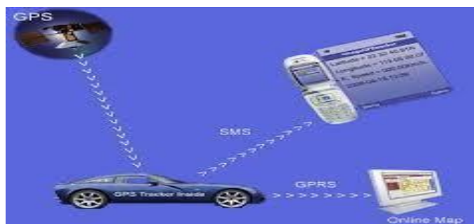
Figure no.1.1 Accident identifier using GPS & GSM
