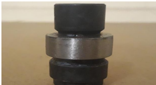
Fig.2.3 Prepared Work pieces after belt grinding.
