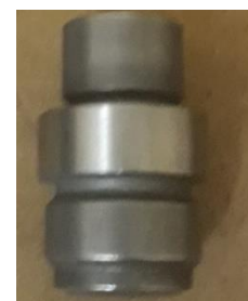
After Heat treatment After shot blasting
