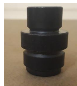
After Heat treatment After shot blasting
