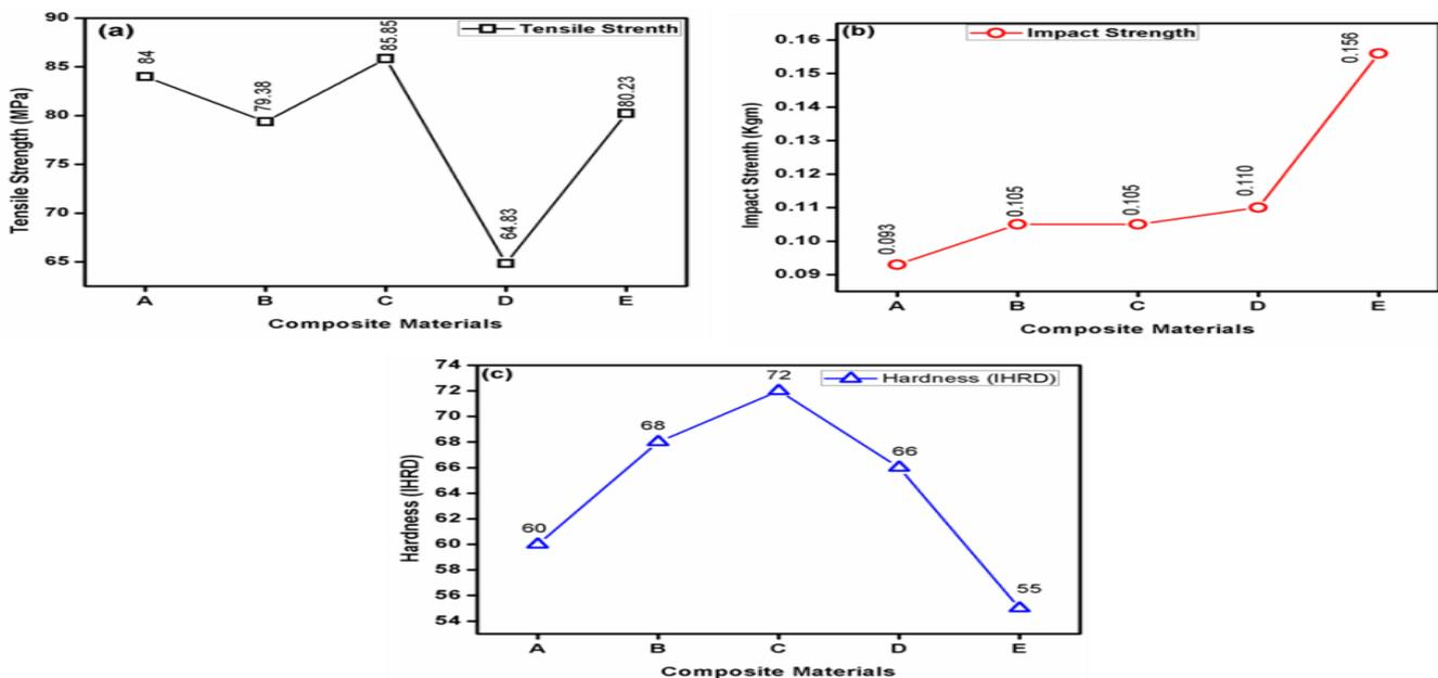
Fig.2 (a) Tensile strength, (b) Impact strength, (c) Hardness strength of composite materials
