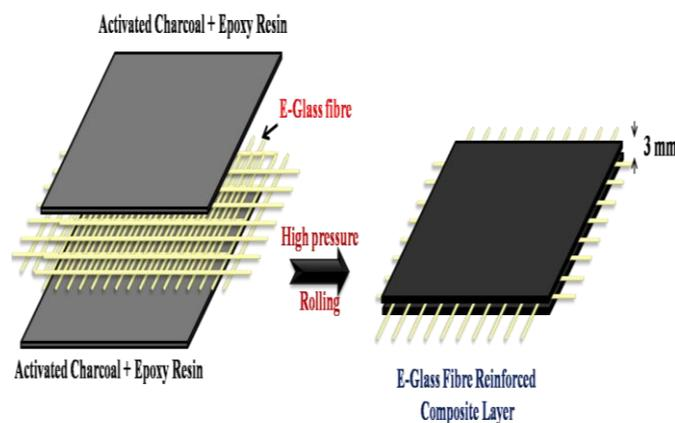
Fig.1 Sample of fabricated material
