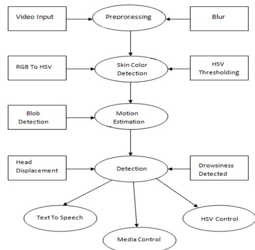
Fig -3: Dataflow diagram
