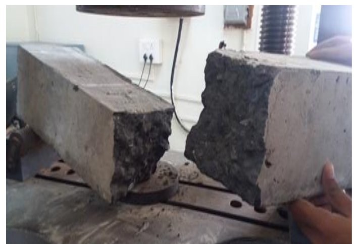
Fig-8: Testing For Flexural Strength
