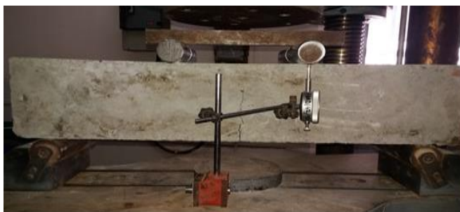
Fig 7: Bending crack in beam
