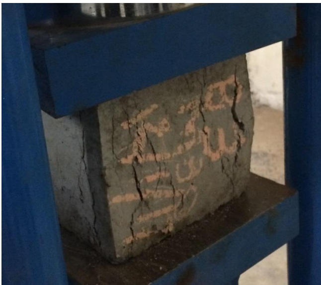
Figure 2: Concrete cube casted with FRC shows higher shatter resistance
