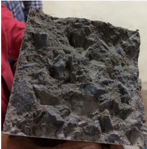
Figure 3: Pull out of coconut fibers. The holes indicate pull out locations
