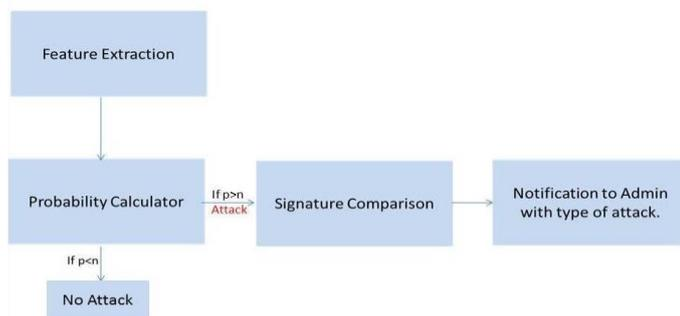
Fig -2: Intrusion Detection Module
