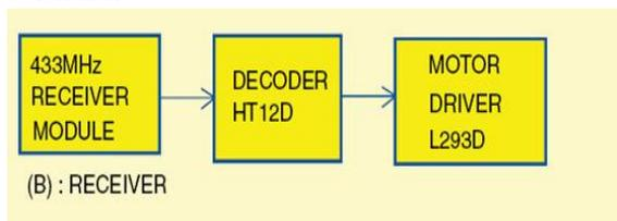
**RF Receiver** of this project will receive the data which is particularly transferred by the transmitter and then on the reception of the received data it transfers it to the decoder.
