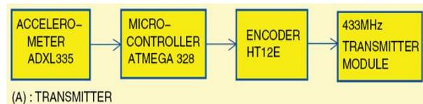
The basic block diagram of the transmitter section of vehicle controlled by hand gesture is shown in the above diagram.
