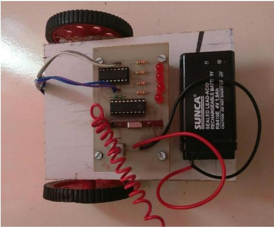
There are two types of RF receiver module. The receiver modules used are super-regenerative modules which are usually of low cost and low power design. They use a series of amplifier and which are used to extract modulated data from a carrier wave. The RF receiver receives the signal from the RF transmitter. Receiver
