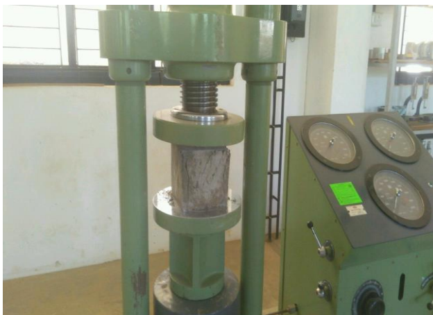
Fig -1: Test setup for cube compressive strength
