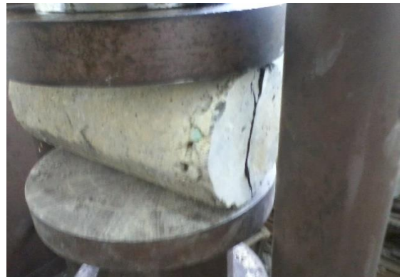
Figure-3 Testing of concrete cylinder specimen
