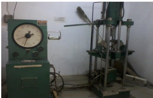
Figure-4 Testing of concrete beam specimen
