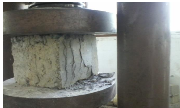
Figure-2 Testing of concrete cube specimen
