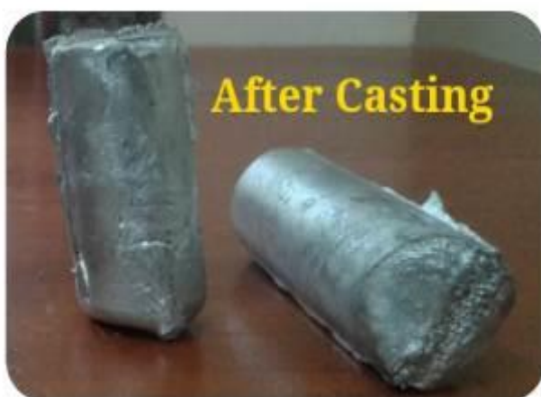
Fig -3: Cylindrical specimens after casting.
